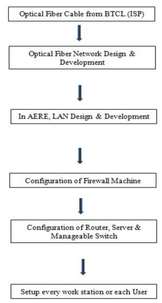
Figure 1: Block Diagram of Whole System Methodology.
